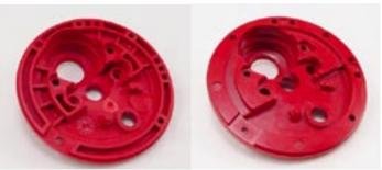
Injection Mold Incorrect Compression Mold Correct
